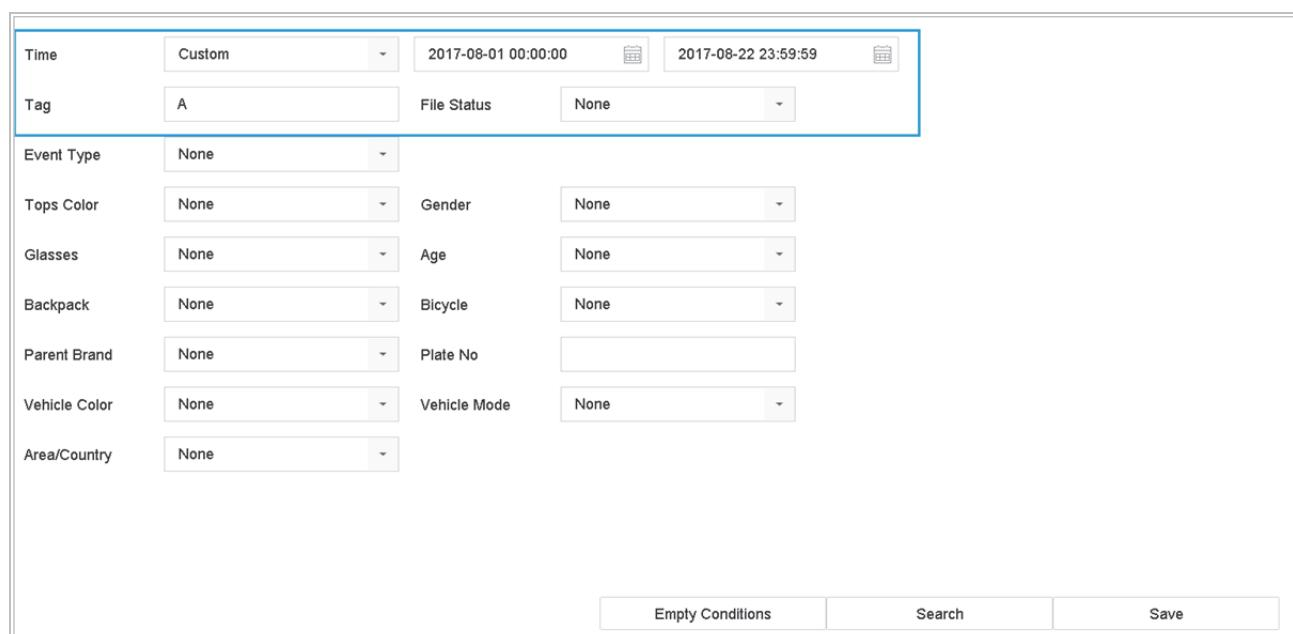
The screenshot shows the 'Tag Search' interface. At the top, there are fields for 'Time' (set to 'Custom' with dates '2017-08-01 00:00:00' to '2017-08-22 23:59:59'), 'Tag' (set to 'A'), and 'File Status' (set to 'None'). Below these are several dropdown menus for filtering by event type, top color, glasses, backpack, parent brand, vehicle color, and area/country. At the bottom right are buttons for 'Empty Conditions', 'Search', and 'Save'.
